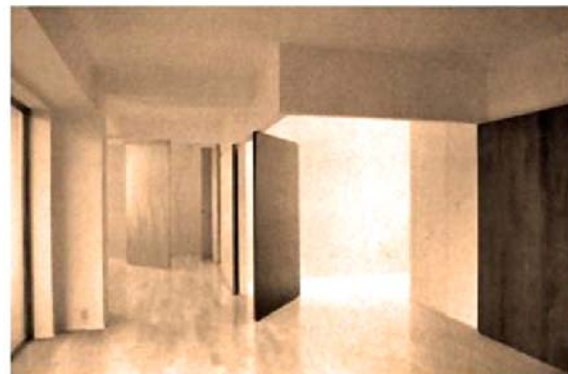
Fig. 47 Hinged walls, closed and opened
