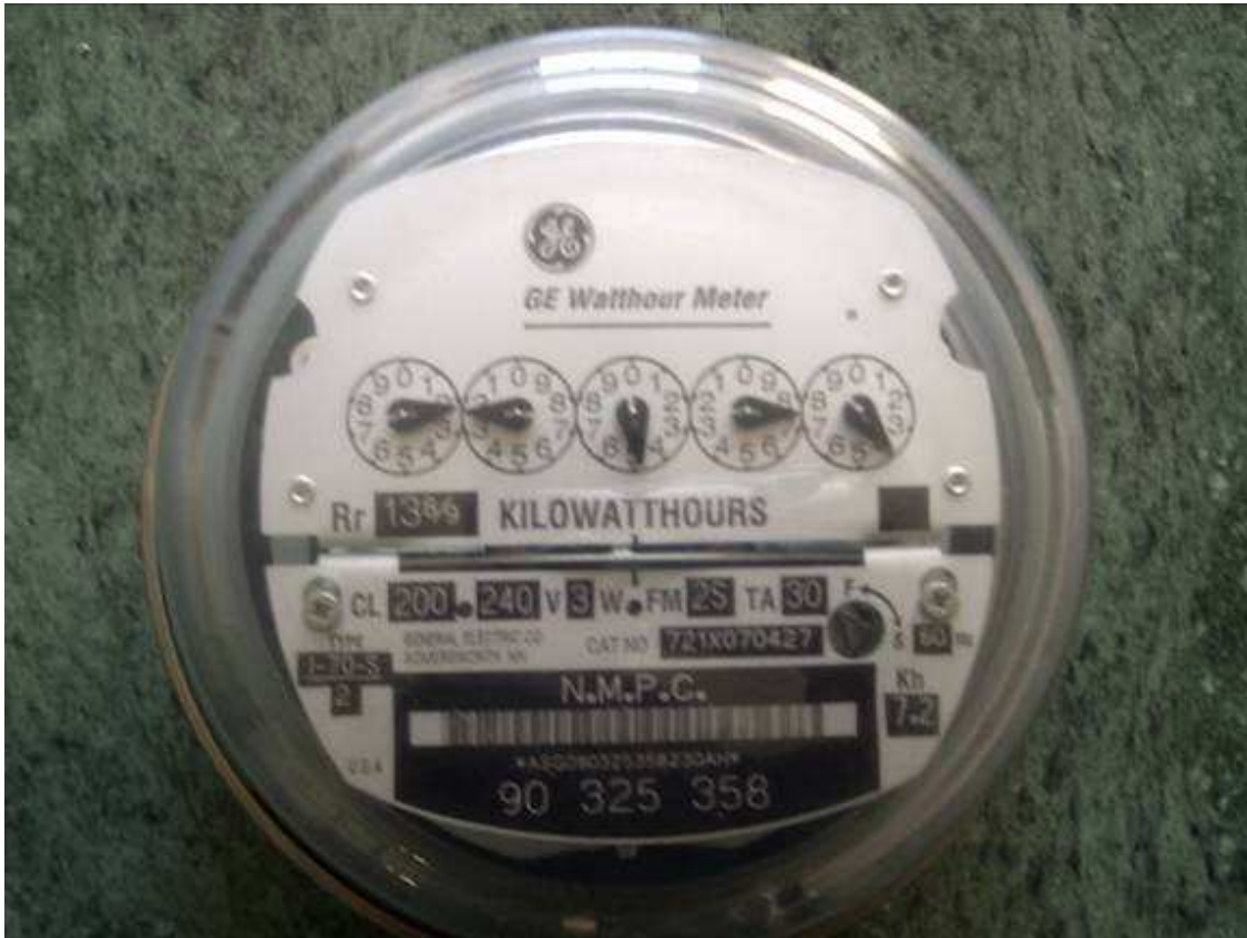
Figure 2.1 Front view of an electromechanical watt-hour meter (Source: www.tdsurplus.com )
