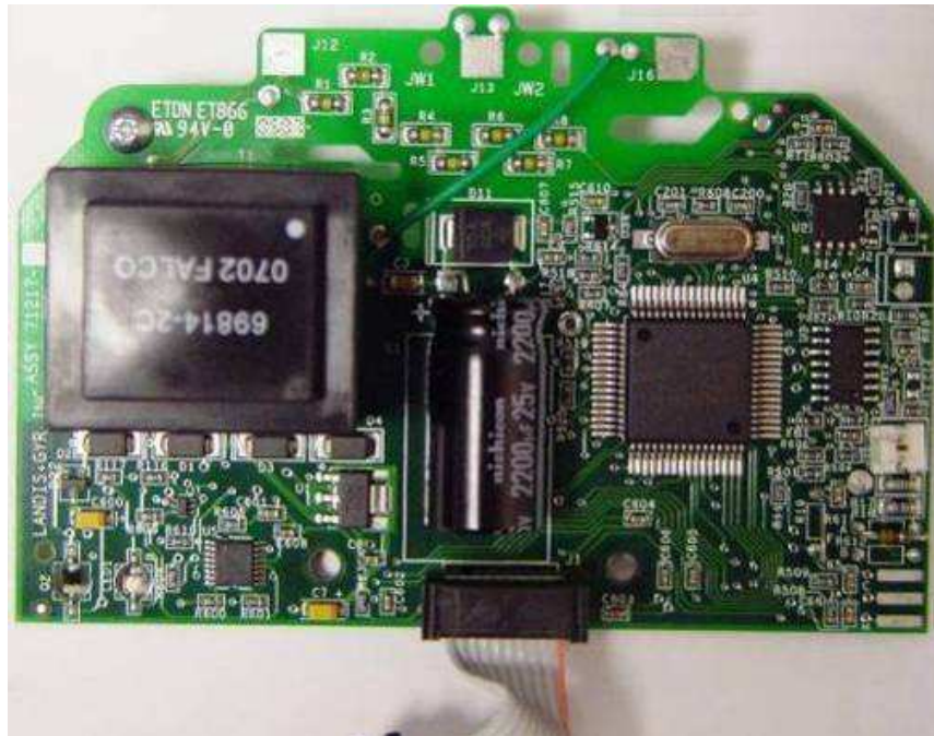
Figure 2.6 Internal components of an electronic watt-hour meter (Landis + Gyr Focus ® meter)
