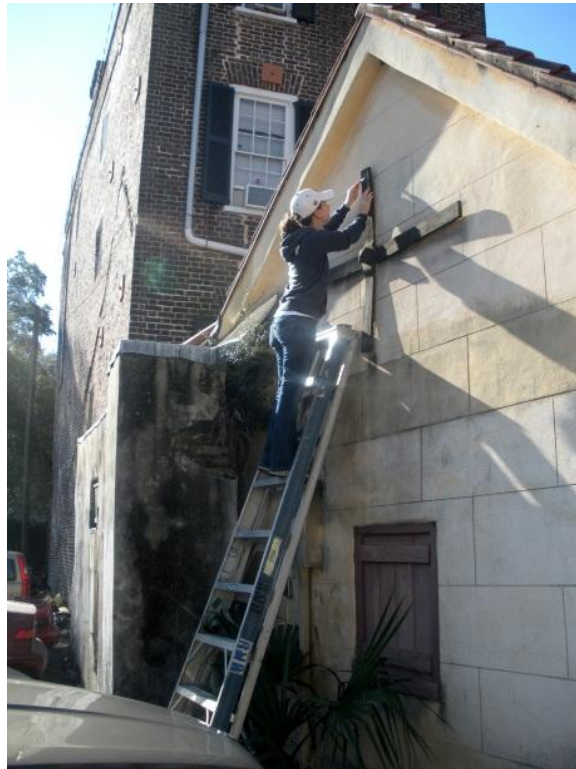
Figure 4.9: Taking a clay mold of the maker's mark on the upper arm of the south-east anchor plate. (Photo taken by student Elyse Harvey)
