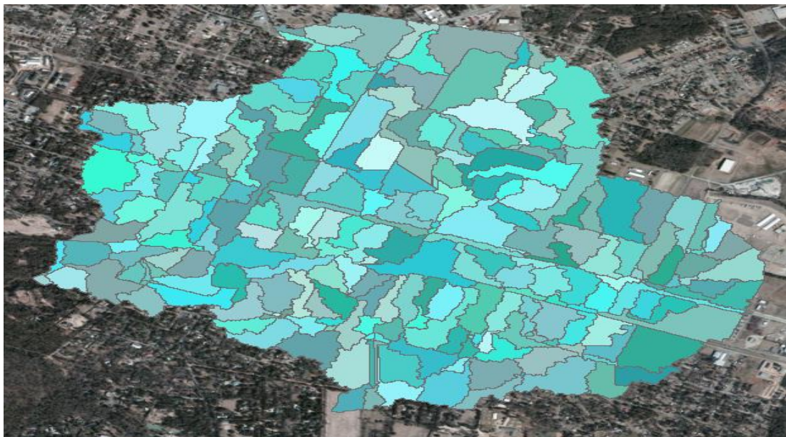
Figure 3.15: Catchment polygon derived from the Stream Link and Flow Direction grids for the 10 foot pipe outlet
