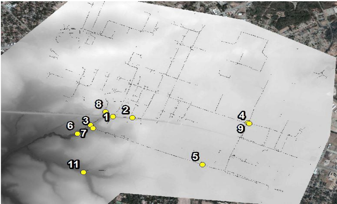
Figure 3.7: DEM after the stormline has been burned in at an artificial elevation and clipped to study area
