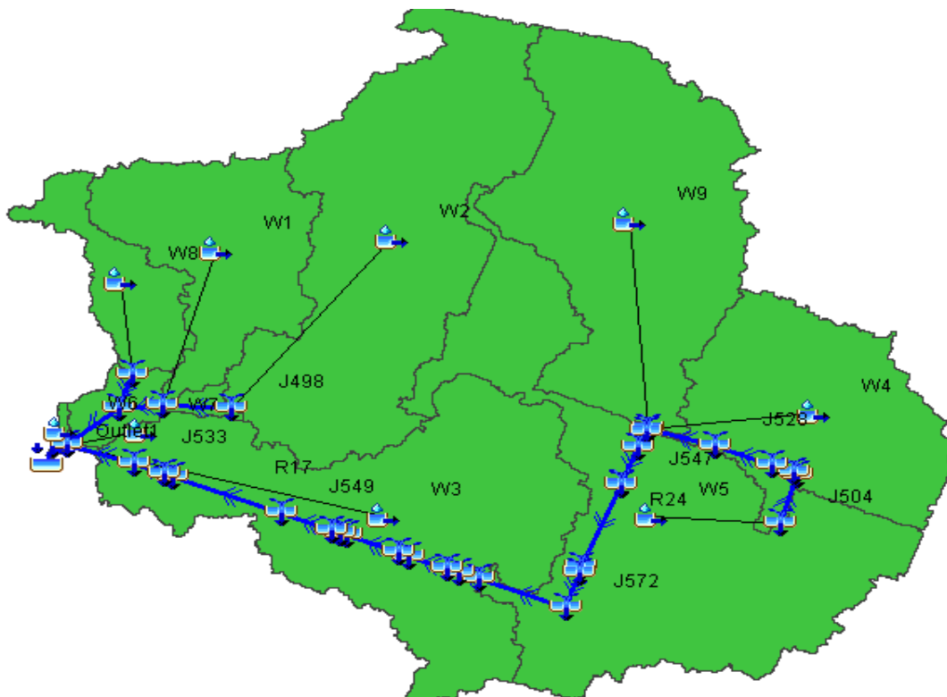
Figure 4.16: HEC-HMS model after export from HEC-GeoHMS and import into HEC-HMS and background shapefile added for illustration purposes
