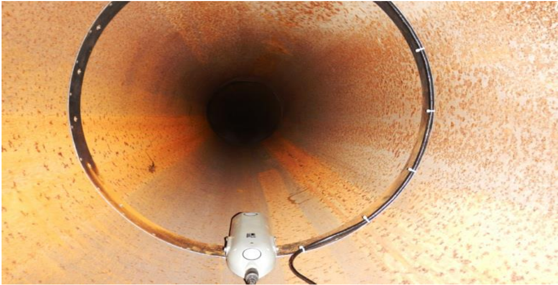
Figure 4.21: SonTek™ Ring mount installed in a pipe with the SonTek™ IQ-Pipe® system (Xylem Inc., 2012)
