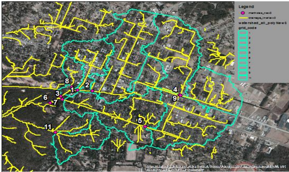
Figure 3.14: Drainage Line created from the Burned DEM showing stormline added to the natural streams
