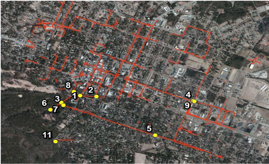
Figure 4.1: Finalized Stormline based on city official drawings and field studies utilized in ArcMap 10.1 and HEC-GeoHMS
