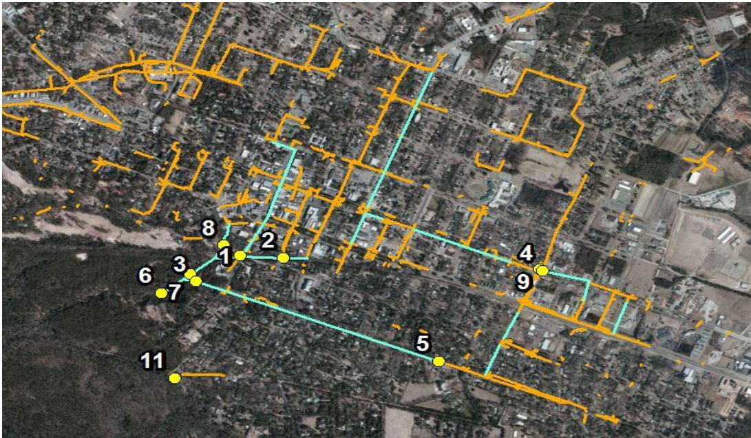
Figure 3.2: Stormline assumptions, in blue, added to the Stormline layer according to project official's hypotheses and field studies
