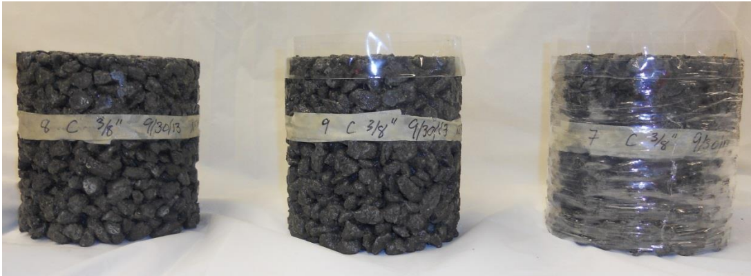
Figure 3.14 Stages in preparing pervious concrete specimens for the permeability test.
