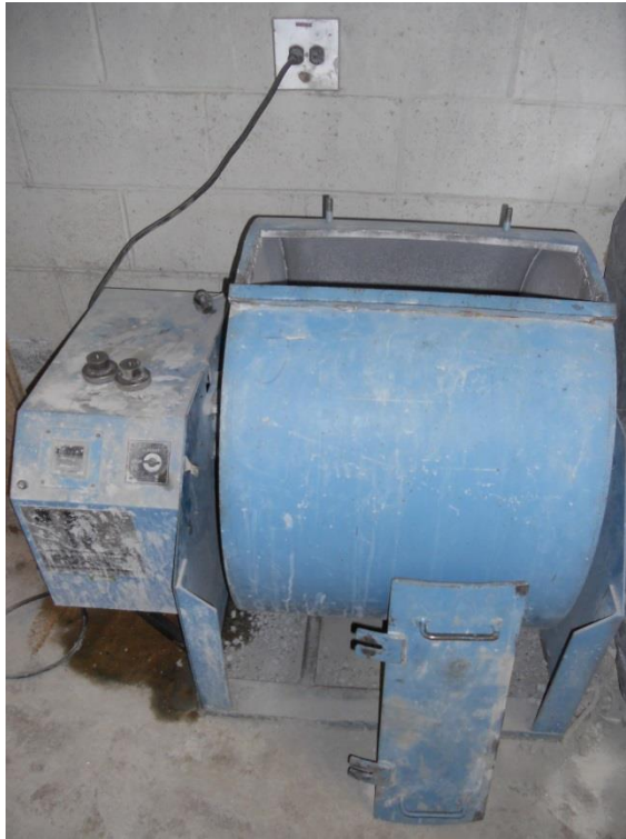
Figure 3.15 LA Abrasion machine used for abrasion loss test.
