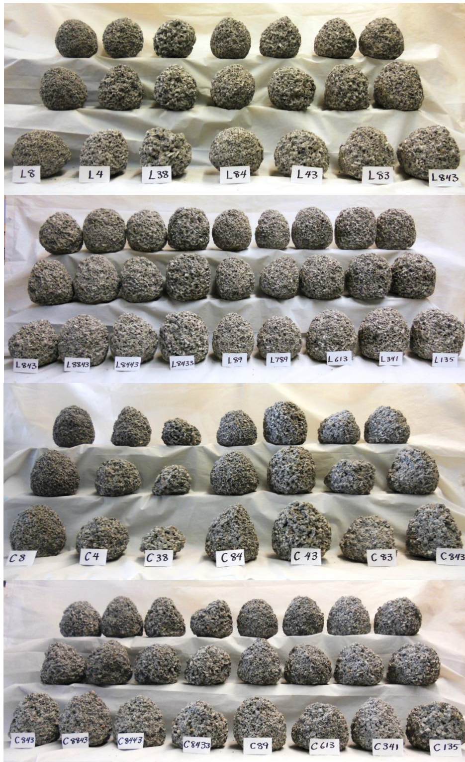
Figure 4.16 PCPC specimens after the abrasion mass loss test for aggregate L and C.
