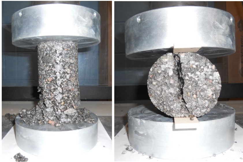
Figure 4.13 Testing PCPC cores made from source C aggregate for compression strength (left) and split tensile strength (right).
