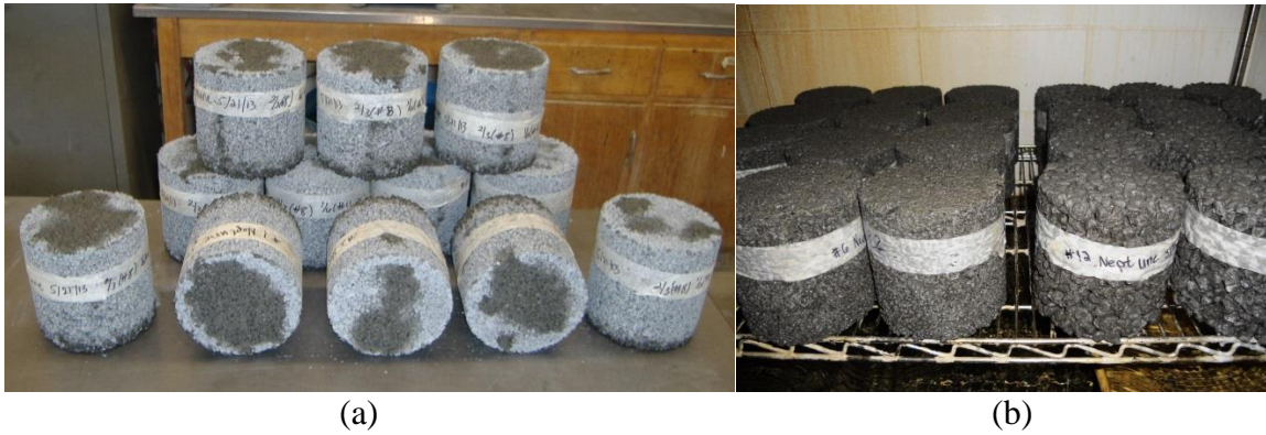
Figure 3.8 Pervious concrete specimens (a) demolded and (b) in wet curing room.
