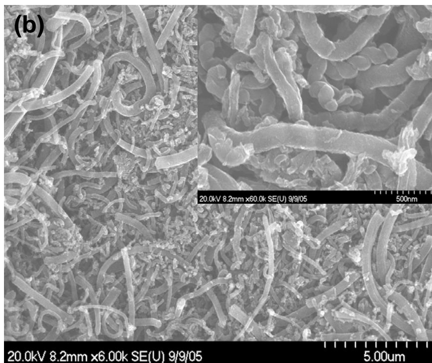
Figure 2.4. Scanning electron micrographs of: (a) PR and (b) MJ fibers.
