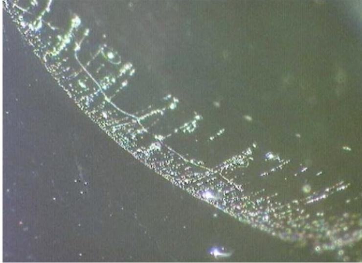
Figure 6.11 Bubble fogs generated during reheat-Pressing of the N-BK7<sup>®</sup> preform that was damaged as result of crack. The length of pattern in above picture is smaller than 2 mm. This picture is obtained from [15].
