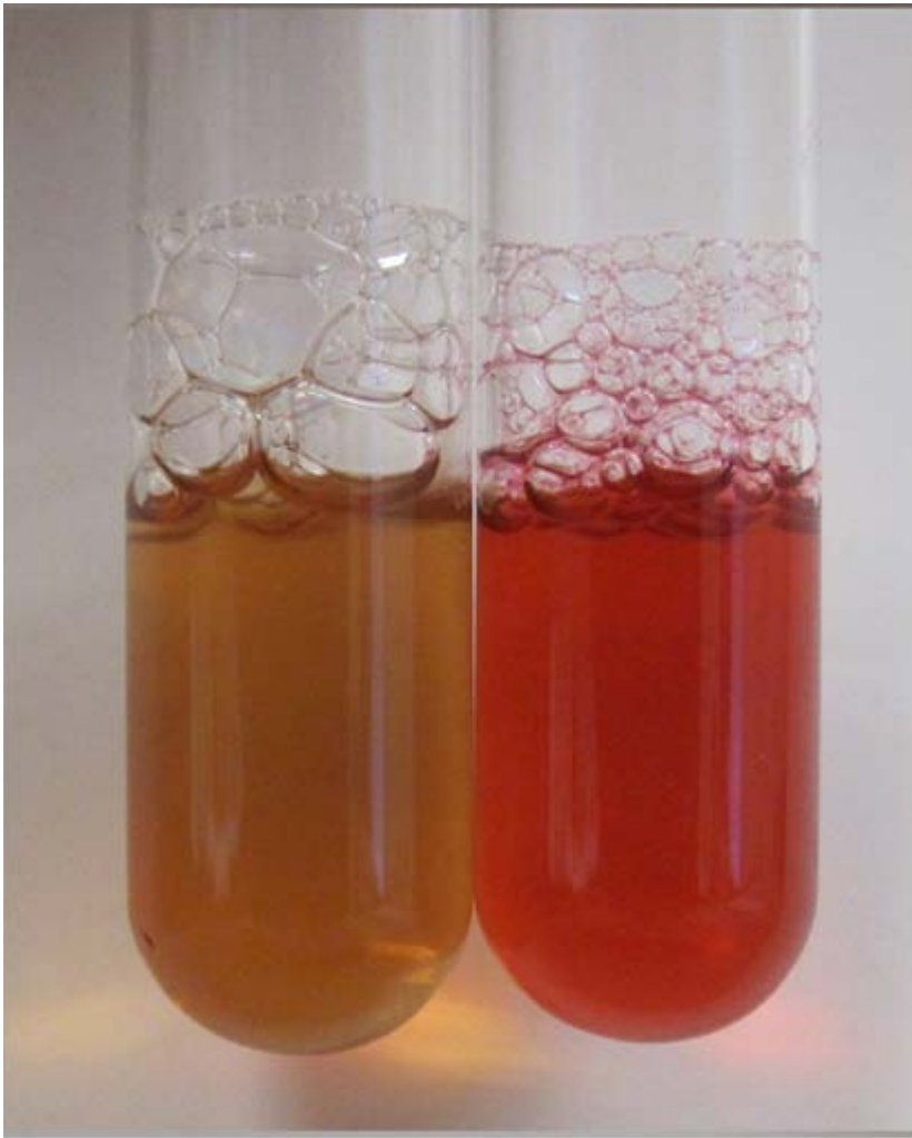
Figure 2.7. Color development in the absence (left) and presence (right) of acetoin upon the addition of a reagent containing 1-naphthol and creatine monohydrate, where the deeper red color indicates a higher level of acetoin. Acetoin concentrations can be quantified by measuring the absorbance at 530 nm in a spectrophotometer.
