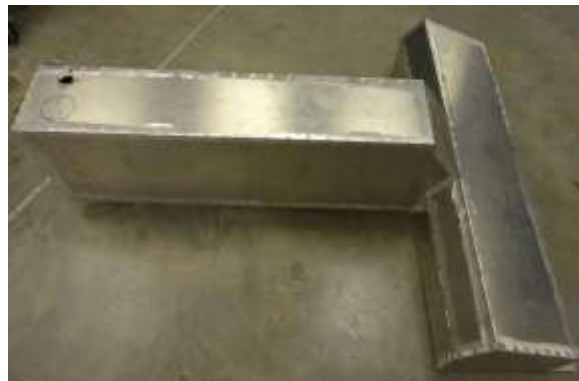
Figure 7.2 Batteries enclosure for electrical vehicle.
