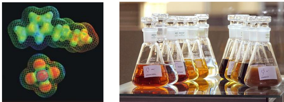
Figure 1.2. Room-temperature ionic liquids (RTILs). Ions in RTILs are often bulky, have complex shape, and feature de-localized charge. Because there exists many types of cations and anions capable of forming RTILs and these ions can be further modified by functionalization, RTILs are considered designer molecules. Left panel: the molecular structure and charge distribution of a popular RTIL 1-Butyl-3-methylimidazolium hexafluorophosphate (BMIM-PF 6 ) 15 . Right panel: different types of RTILs showing different colors 16 .
