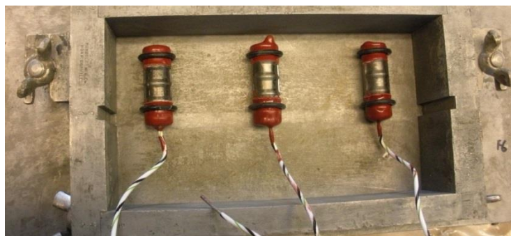
Figure 4.4.3 Position of steel bars at the bottom of the mold
