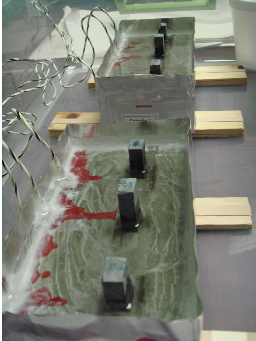
Figure C.2. Sample with chloride reservoir of top of it
