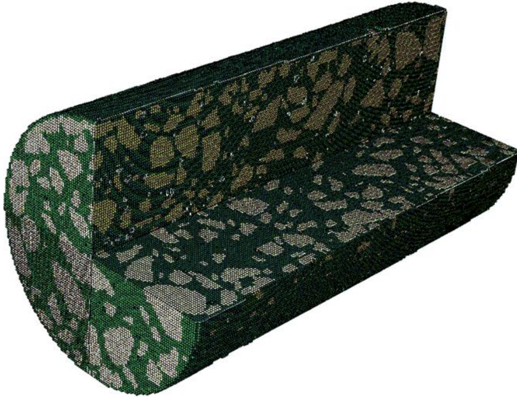
Figure A3. Sectioned view of concrete 3D finite element model (Coarse mesh 1 \times 1 \times 1 \text{mm}^3 )
