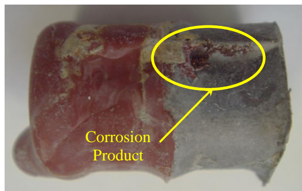
Figure 4.4.10. Corrosion on the surface of the steel bar with 3mm distance to the aggregate
