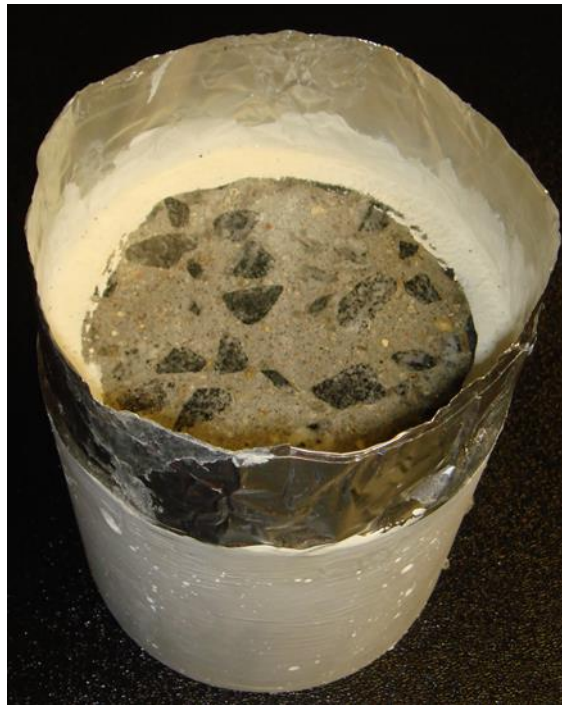
Figure 4.3.1. A sample with chloride solution ponding placed on the top of it
