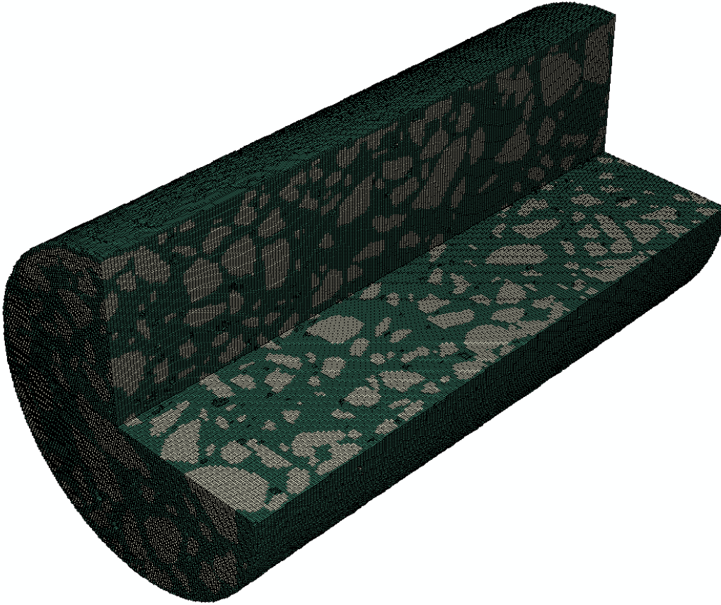
Figure A2. Sectioned view of concrete 3D finite element model (Fine mesh 0.5 \times 0.5 \times 1 \text{mm}^3 )
