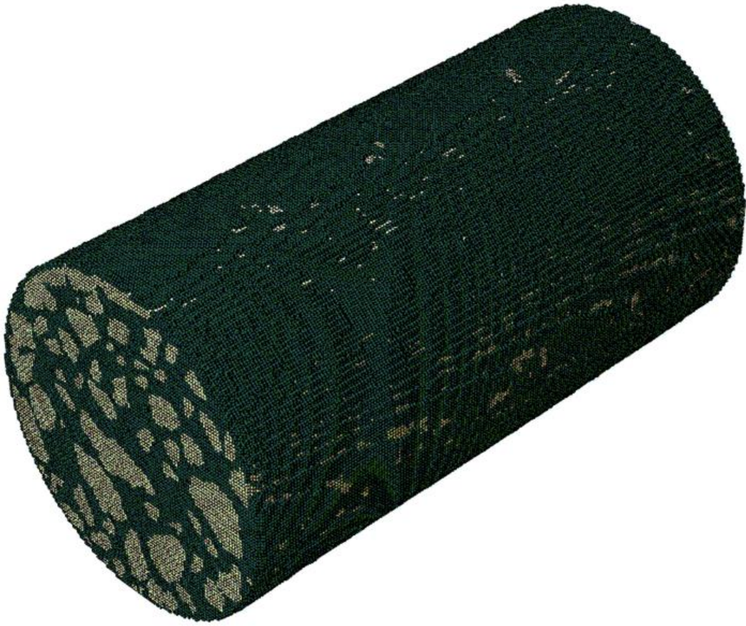
Figure A1. Concrete 3D finite element model
