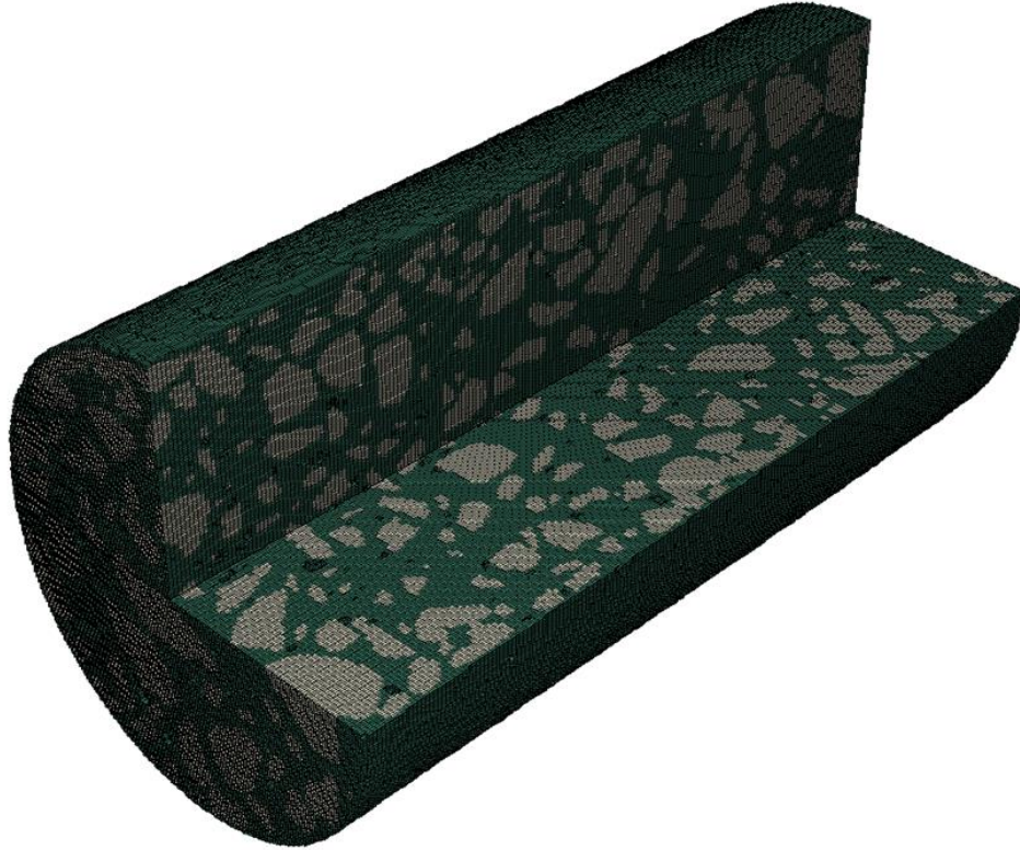
Figure. 3.2.3.2 Three-dimensional FEM of one of the cylinders
