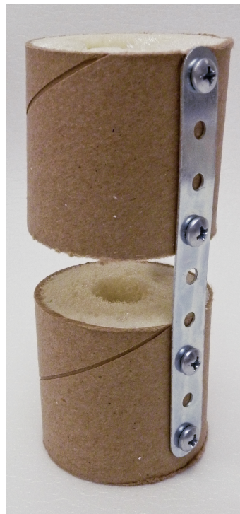
Figure 4.3. Example of fracture repair of simulated bone fracture with ~1 inch gap for testing.
