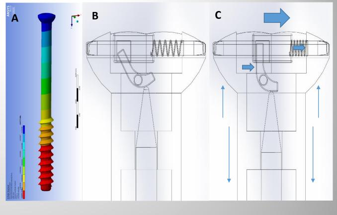
$\succ$  The spectral rulers developed can be easily  $\succ$  Prototype 4 design for orthopaedic screws to help obtain mechanical advantage of ~10 and thus improve sensitivity of the spectral rulers.
