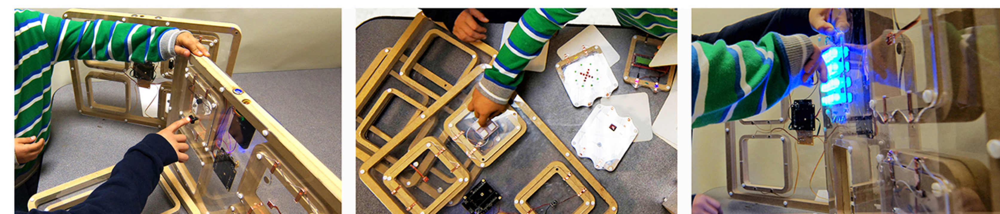
Fig. 9: CyberPLAYce (Prototype A-1) - Our scenario unfolding... LEFT: Push the button on the Buzzer module to turn the alarm off. CENTER: Push a button on the 2x2 Button-Light Module to turn the bedroom light on. RIGHT: Push a button on the 4x4 Button-Light Module to turn on the rainbow.
