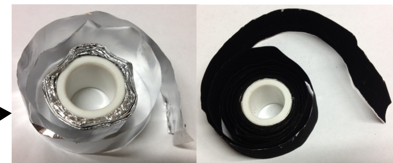
Al foil rolls before and after CNT growth
