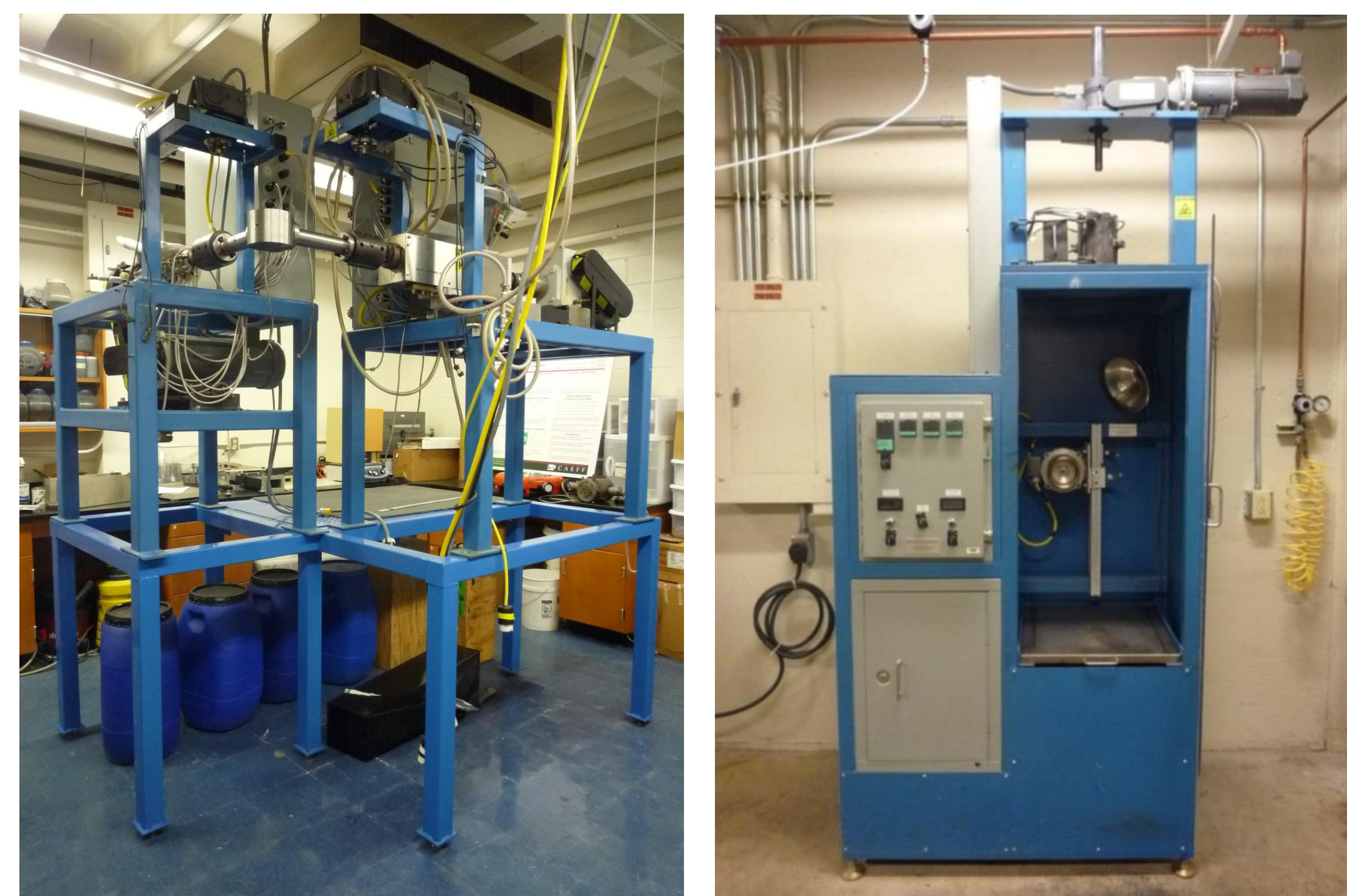
Left: Alex James@ bicomponent spinning device. Right : Alex James@ batch melt spinning device.
