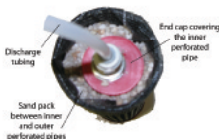
Exploded endview of sampler
