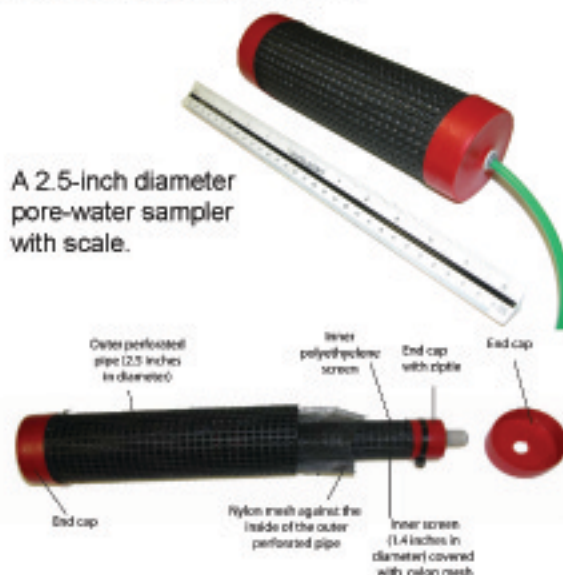
Lengthwise exploded view.
