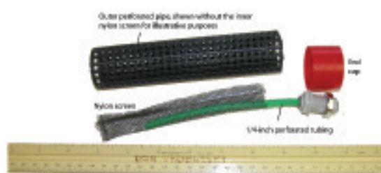
Exploded 1.4-inch diameter sampler
