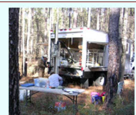
A Geoprobe drilling rig was used for coring and well installation – it is lightweight for use on soft soils, can access wooded areas, and allows for rapid assessment of geology.
