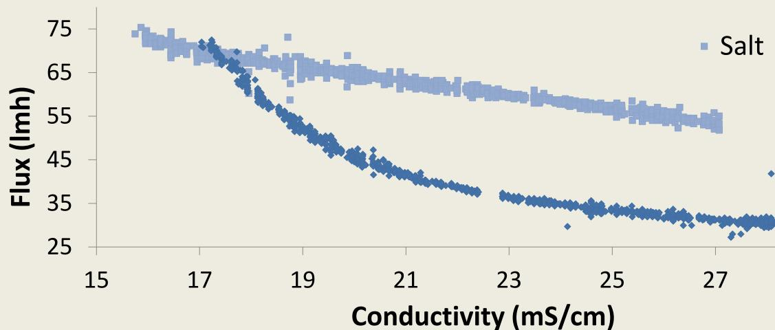
Figure 3: An example of a scaling experiment. NaCl does not produce scales and flux decline is linear with increasing concentration. In scaling solutions, flux decreases both due to increasing concentration and scale formation.
