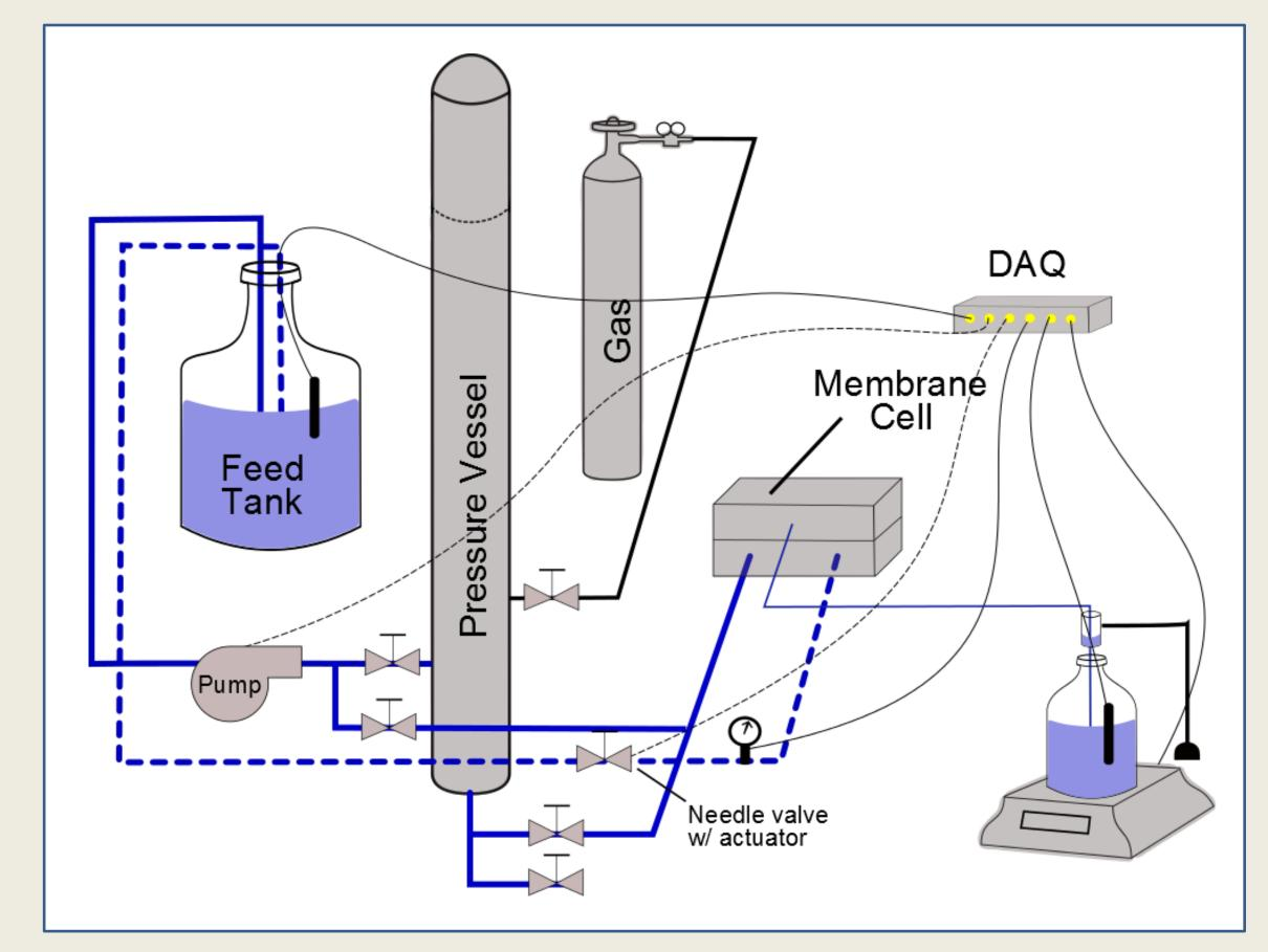
Figure 2: Sketch of bench-scale testing apparatus.
