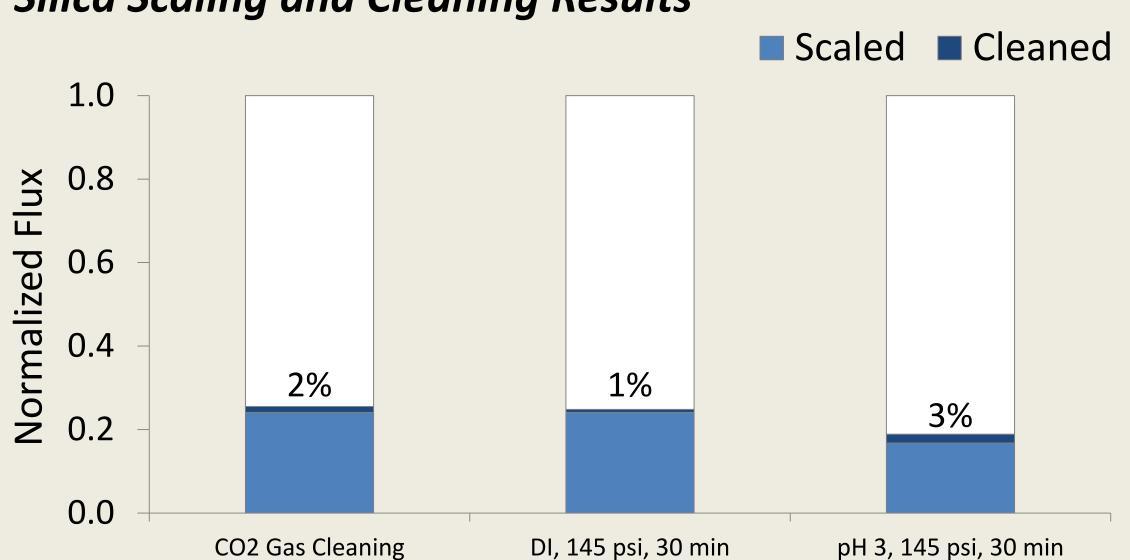
Figure 5: Comparison of cleaning efficiencies for membranes scaled by silicates. None of the attempted cleaning procedures regenerated flux.
