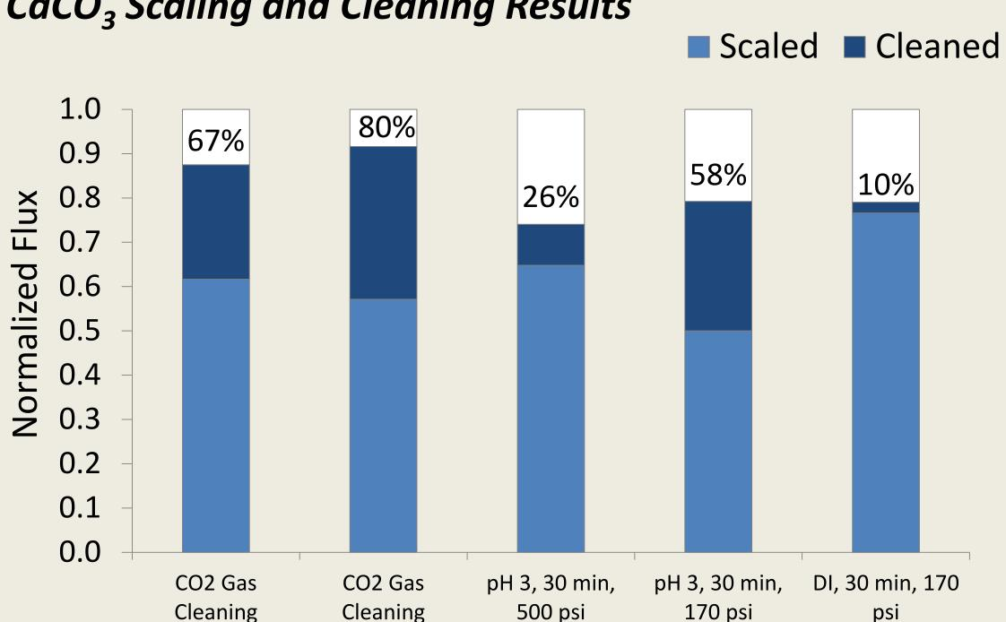
Figure 4: Comparison of cleaning efficiencies for membranes scaled by CaCO<sub>3</sub>. Cleaning with dissolved CO<sub>2</sub> returned the most flux, followed by acid cleaning.
