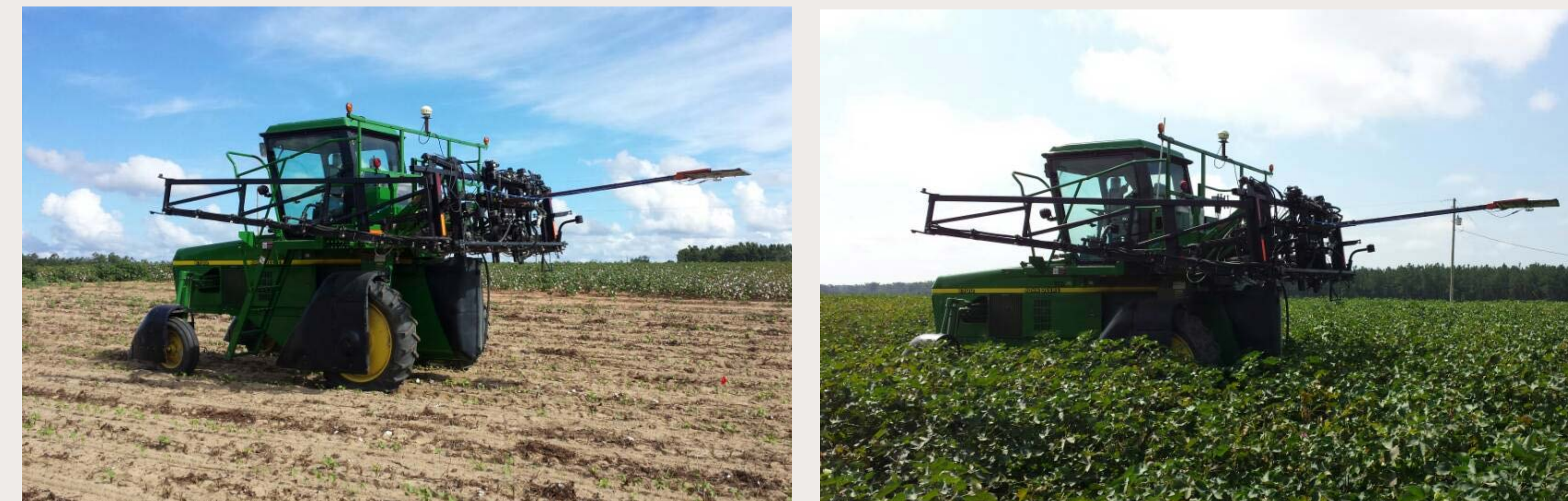
Figure 4. Hi-boy mounted DMR collecting data from bare soil (left) and cotton field (right).
