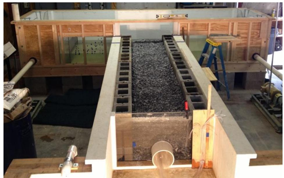
The flume used had a 3 m test section. The inflow was controlled by 2 pumps with variable frequency drives and the flow rate was measured by 2 v-notch weirs. The pressure was measured along the pipe using piezometer tubes.
