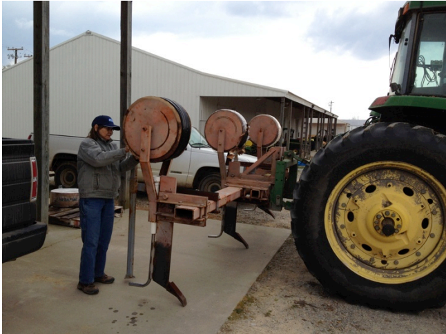
Figure 3. Shank system used to install the drip tapes.
