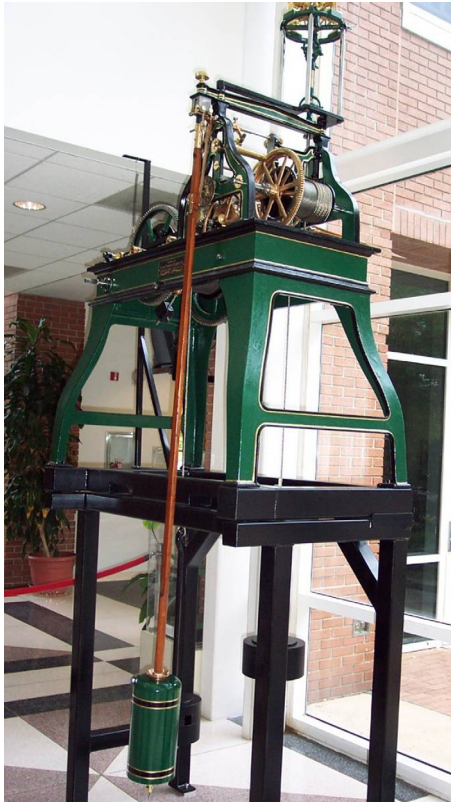
Fig. 1. 1905 Seth Thomas tower clock at Clemson University mounted on a pedestal with pendulum and clock face assembly.
