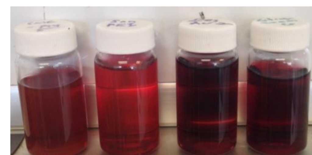
Image of various types of GNPs: (Left to Right) CMC, 5nm PEI, PEG, Citrate 20 nm
