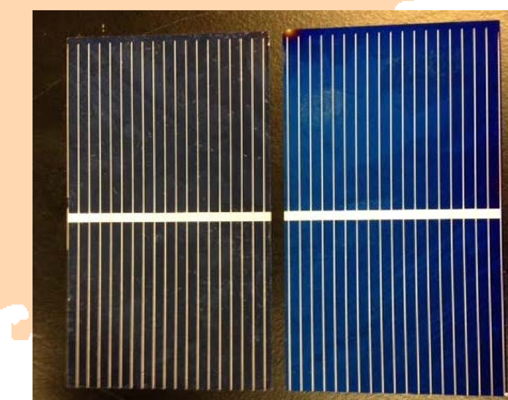
Figure 4: Solar Cells from RadioShack. Coated with Acrylic Spray Coating(left) and uncoated.(right).
