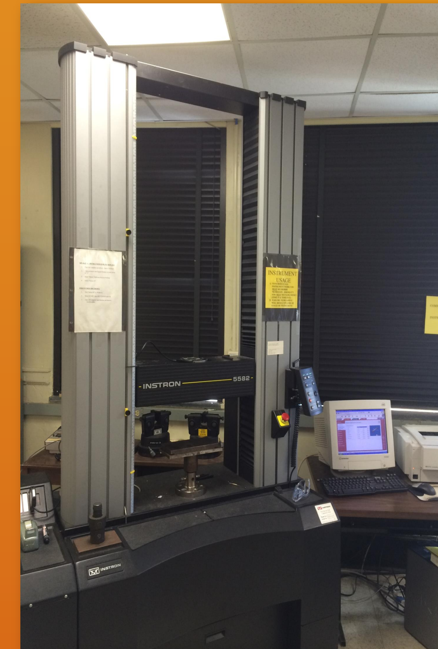
Above Right: Instron machine used for testing material properties like hysteresis
