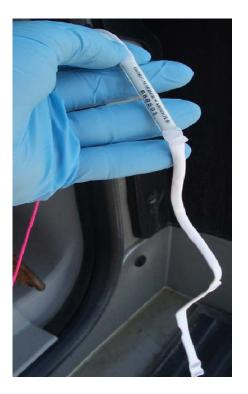
Figure 2. The GORE<sup>™</sup> Module ready to be installed in a shallow borehole in the field.
