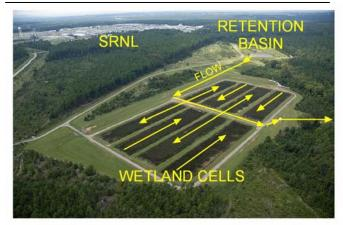
Figure 1. Layout and water flow path through CWTS for A-01 outfall.
