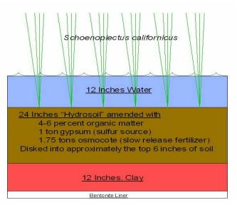
Figure 3. Typical cross section of wetland treatment system.
