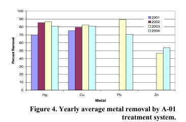
that is now available. Because the design of the system encourages a low redox status of the sediments in the treatment cell, it was anticipated that mercury would also be removed from the water column. Mercury removal improved with maturation of the vegetation and the sediments, and averaged greater than 80% removal of total mercury during the second year of operation and was below the new permit limit.
