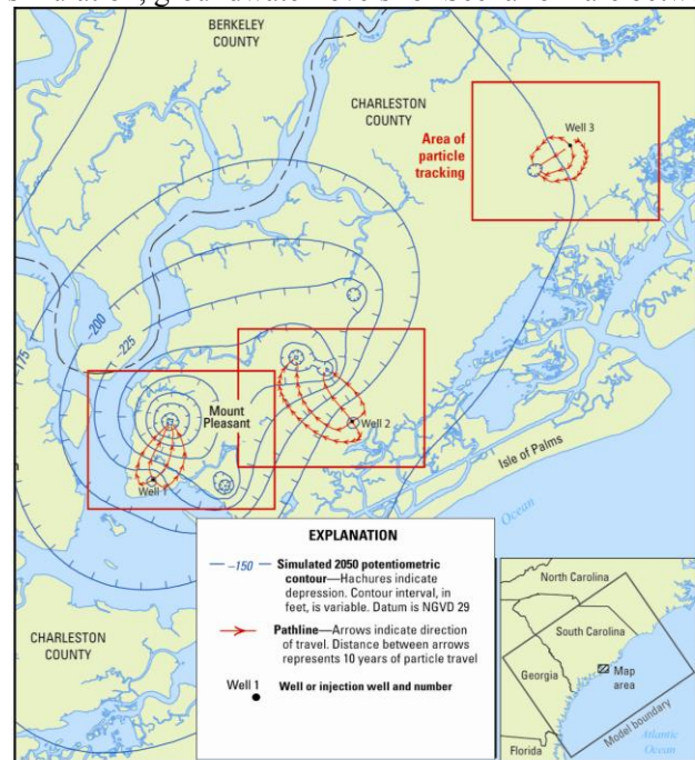
Figure 1. Simulated 2050 potentiometric surface map of the Middendorf aquifer near Mount Pleasant, South Carolina, and particle-tracking results using a 30-percent porosity for Scenario 2 for particles released at three proposed injection wells.
