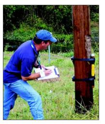
Figure 2. Water-level sensor device attached to power pole.
