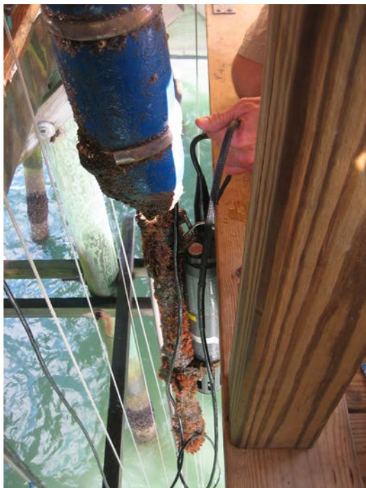
Figure 2. Pier monitoring station at the Second Avenue Pier showing ziplines and counterweighting. (a) Left photograph shows the surface sonde strapped to a PVC “sled” that slides vertically on the ziplines. The blue buoy is flotation that maintains the surface sonde’s position about 1 m below the sea surface. (b) Right-hand photograph shows the zipline and PVC sled. The blue box in the upper left corner houses the RAD-7 detector. Red hoses in the lower right-hand corner are part of a filter manifold that prevents particles from clogging the Rn detector.
