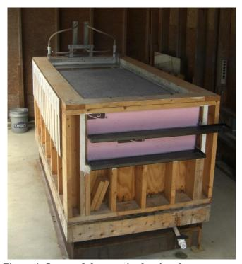
Figure 1: Image of the test rig showing the pavement, weir, manometers for measuring subsurface flow, and the collection trays at the downstream end.
