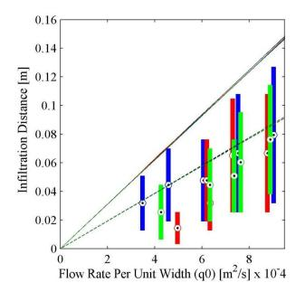
Figure 3: Plot of measured infiltration distance versus flow rate for pavement slopes of 0% (blue), 5% (red), and 10% (green). The solid line represents model results for hydraulic conductivity, K, equal to 0.0064 m/s, and the dashed line represents K equal to 0.0103 m/s.
