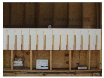
Figure 2: Image of calibration testing. Red food coloring has been used to enhance the resolution of the water level inside manometer tubes. Photos were taken at 30 second intervals to determine the change in depth of water within the aggregate layer over time.
