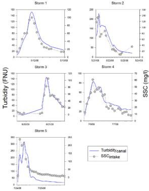
Figure 3:Turbidity and SSC for 5 storms at Crabtree Canal.
