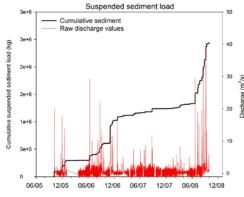
Figure 7: Estimated suspended sediment loading over the period of available data at Crabtree Canal.
