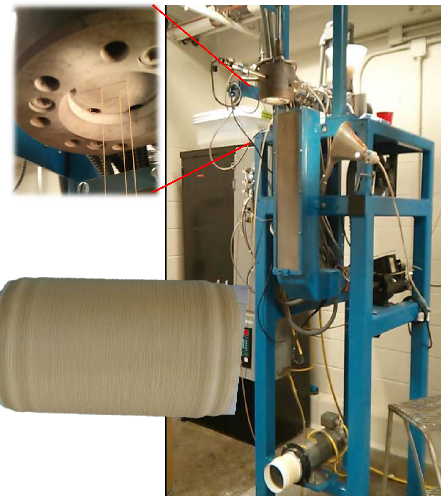
Alex-James spinning unit ( 1.3 m ) and the spool of soy-PE fibers . Average fiber diameter was 52 \pm 4 \mu m or 22 denier with a draw down ratio (DDR) of 92
