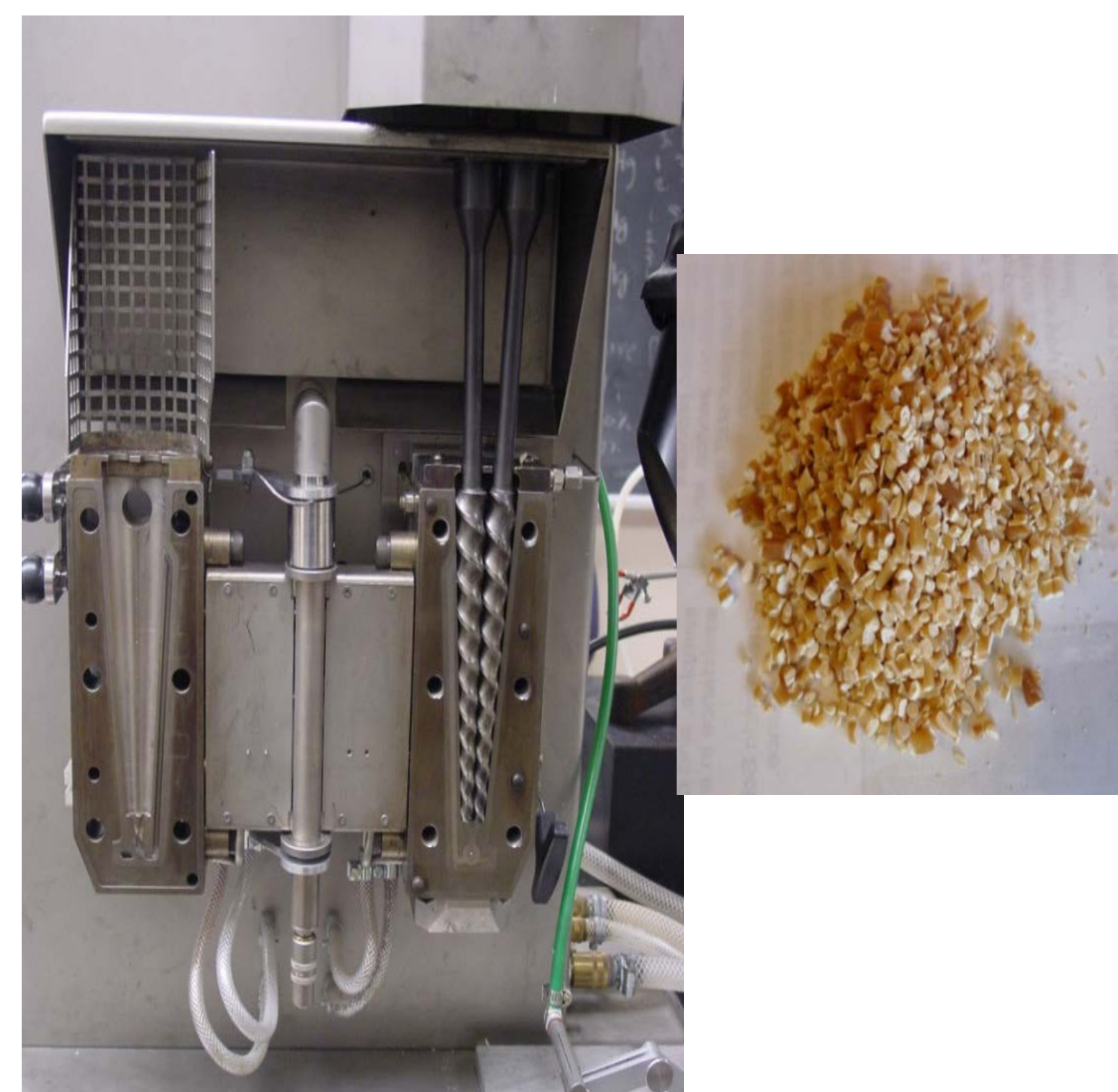
DSM micro extruder was used for dispersion of soy flour in PE matrix and the production of PE-soy pellets. The micro-extruder has a recirculation channel and was operated in semi batch mode.
