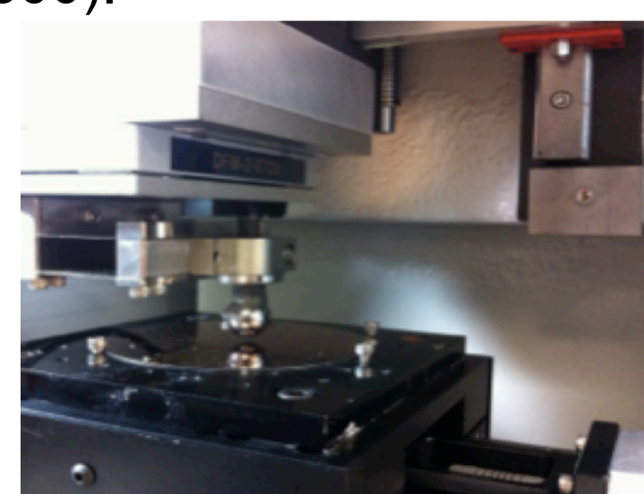
Fig. 2 Linear reciprocating wear test of Cu/Nb nanolaminate and stainless steel counterface.
