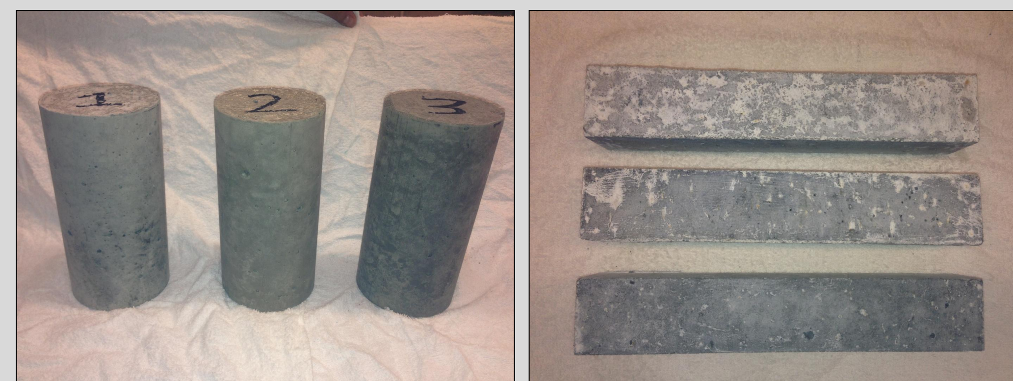
Figure 3: Concrete specimens for strength and durability tests
