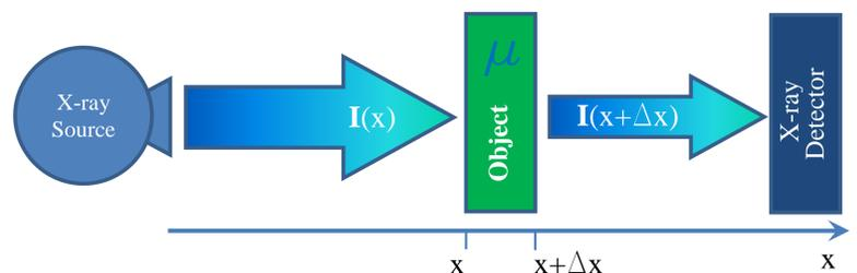
Figure 5. X-ray attenuation mathematical model while running through a homogeneous object with constant attenuation  $\mu$
