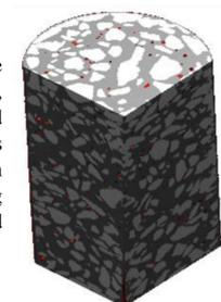
Figure 17. Inside sectioned view of 3D model of concrete sample.
