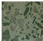
Figure 4. Real aggregates have non regular shape
