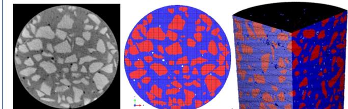
Figure 15. A slice of concrete QCT image including coarse aggregates, voids and concrete matrix together with finite element model corresponding to the same slice.
