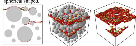
Figure 3. 3-D tensile damage propagation of cementitious composites<sup>3</sup>.
