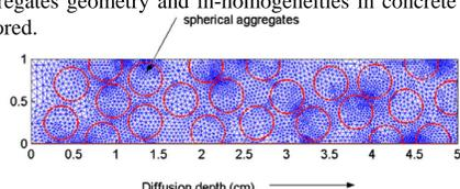
Figure 1. Model of concrete for diffusion with circular aggregates<sup>1</sup>.
