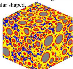
Figure 2. 3D image of hydrated cement paste<sup>2</sup>
