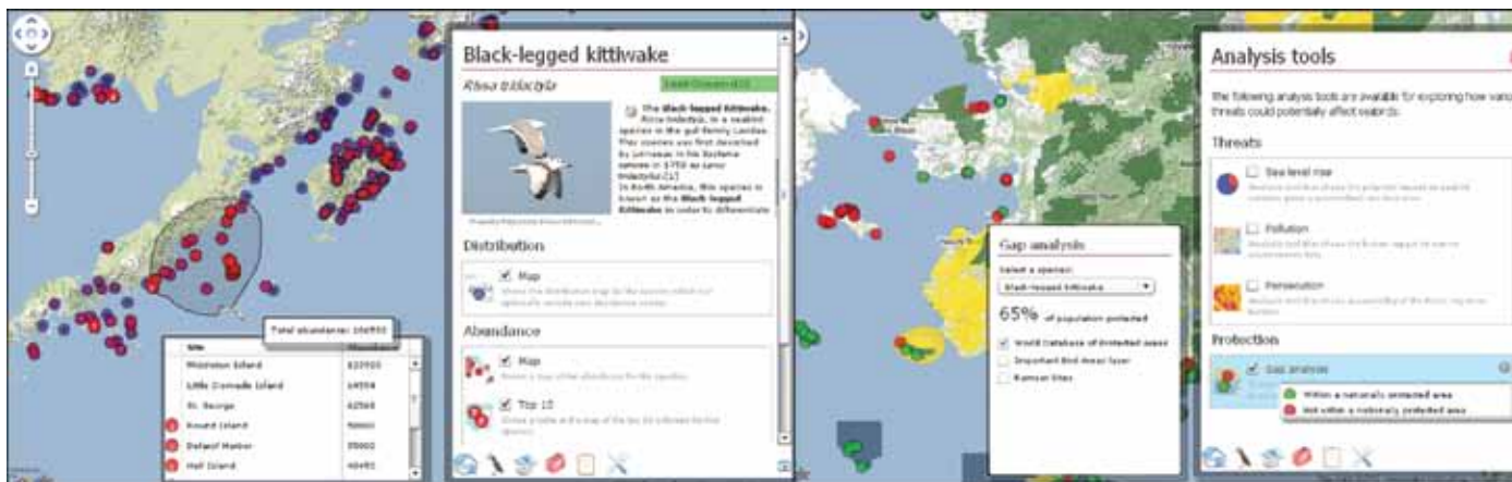
Fig. 3.9-3. Screenshots of the CBMP data portal. On the left are population data locations and summary information being provided from a distributed data node. On the right is an example of an analysis tool that indicates where a seabird colony is located as it relates to various land-use designations.
