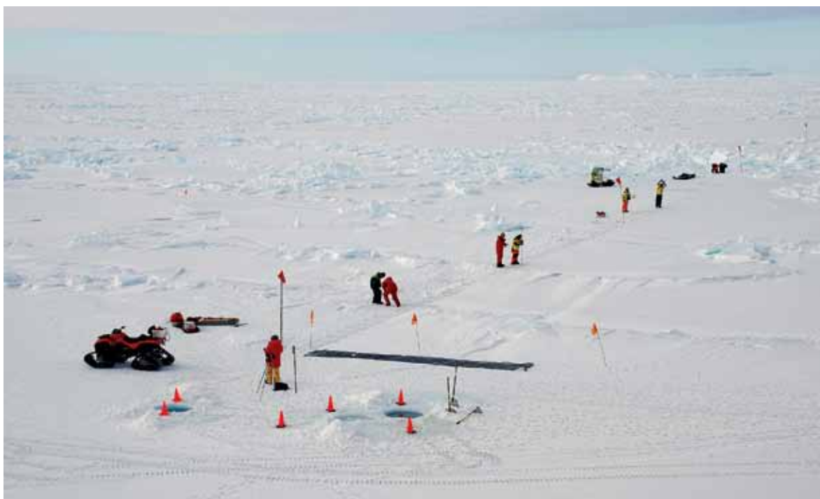
Fig. 2.3-13. An ice thickness transect across an ice floe in East Antarctica out during the IPY project SIPEX onboard Aurora Australis, between 110°E and 130°E in September-October 2007. Sea ice and snow cover thickness were measured in situ and related to aircraft measurements. The black strip at the beginning of the transect is mesh sheet that acts as a radar reflector for the aircraft.
