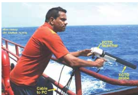
Fig.5.3-5. The data collection campaign for IPY project no. 70 launched in austral summer 2007. Project PI, Alvarinho J. Luis launches an XCTD probe in the Southern Ocean.
