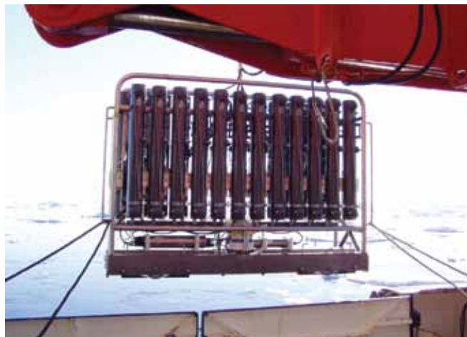
Fig. 2.2-7a. Ultrapure all-titanium frame holding 24 teflon-coated water samplers of 12 Liters each, deployed with a Kevlar cable. Upon recovery the complete frame is placed inside an ultraclean room for subsampling. The frame never touches the steel ship and thus permits reliable sampling of ultralow concentrations of dissolved Fe in pristine ocean waters.
