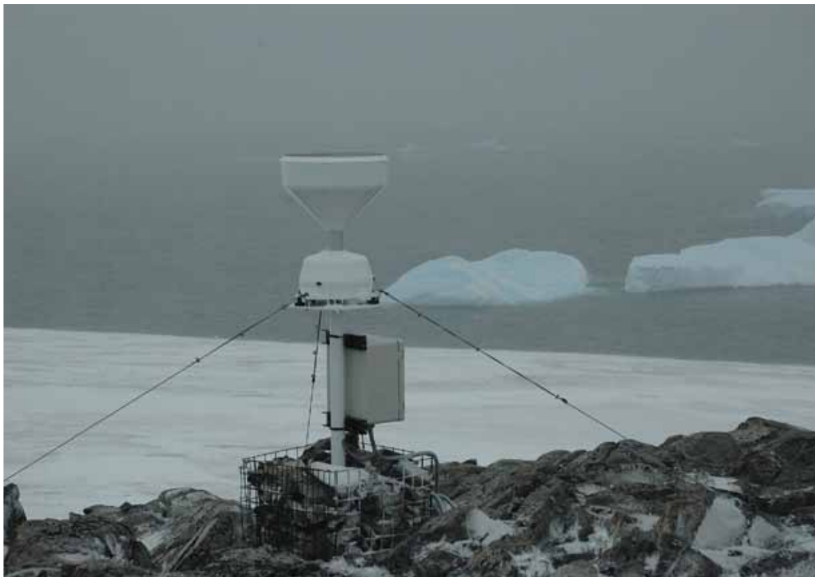
Fig. 3.5-5. A modern aerodynamic automatic tipping bucket gauge at Rothera (U.K.). It doesn't work well in Antarctica, particularly in light snow or strong wind, and needs a shield.
