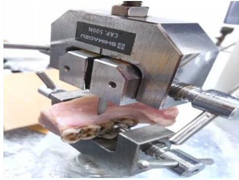
Figure 1. Mounting in the texture analyzer to measure shear force in a pig mandible (lateral view).
