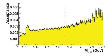
FIG. 8. (Color online) Acceptance of CLAS versus the invariant mass of the  $\Xi^-\pi^-$  system, determined from the  $\gamma d \to K^+K^+\Xi^-\pi^-p_s$  phase-space simulation using a GEANT-based detector simulation package GSIM. The red vertical line indicates the position of the peak seen by the NA49 collaboration.
