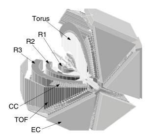
FIG. 1. Three-dimensional view of the CLAS, showing the three regions of drift chambers (R1–R3), Čerenkov counters (CC), the time-of-flight system (TOF), and the electromagnetic calorimeter (EC) (see text for details). In this picture, the photon beam travels from the upper-left corner to the lower-right corner.
