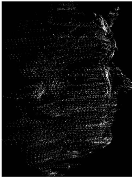
Fig. 14 Raw data cloud of a live subject using the dual tracker that allowed free head movement.
