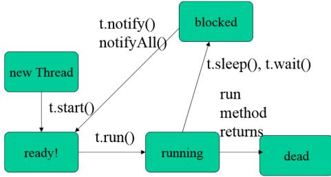
Figure 1. The Life Cycle of a Thread
