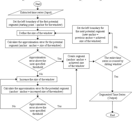
Figure 8. The flowchart for the Sliding Window algorithm
