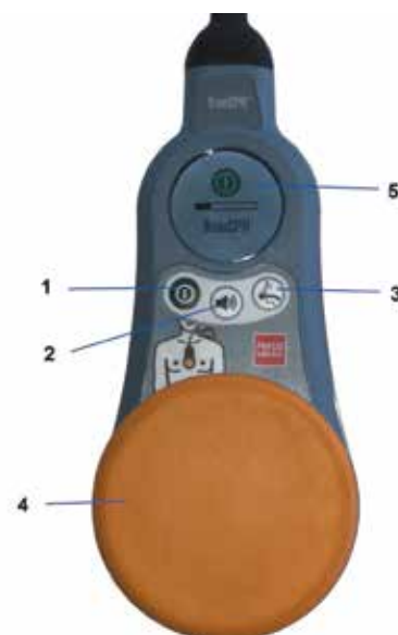
FIGURE 4. Construction of the chest overlay of the TrueCPR device. Legend: (1) on/off button; (2) mute button; (3) change of mode in the case of an intubated patient; (4) hand pad; (5) display of resuscitation parameters
