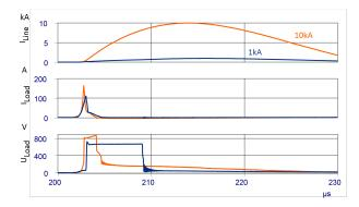
Figure 4. Behaviour of the arrangement in case of transient currents 1 kA (blue) and 10 kA (orange)  $8/20 \,\mu s$ top - transient impulse line current; middle - transient impulse load current after switch; bottom - load voltage
