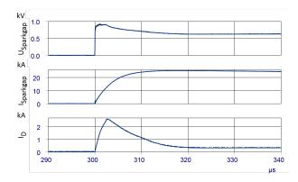
Figure 7. Behaviour of common triggerable spark gap during a lightning current of  $25 \text{ kA} \ 10/350 \ \mu s$  top voltage spark gap and consumer, middle - impulse current spark gap, bottom - impulse current load / consumer in case of an varistor (S20K275) within the consumer
