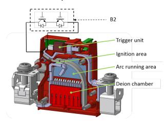
Figure 5. Spark gap with trigger unit and additional actuation by B2
