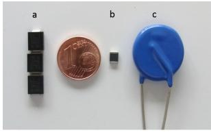
Figure 8. Picture of suitable overvoltage protective components for use as secondary protection D or within consumer C by use of the tested arrangement a - suppressor diodes; b - SMD varistor; c - normal varistor S20K275
