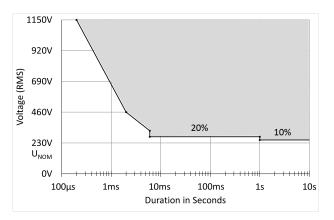
Figure 1. Voltage tolerance curve proper for 230 Volt AC equipment
