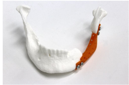
Fig. 5: 3D Printed models of a) mandibular implant and b) mandibular implant positioned and fixed on the mandible and TMJ.
