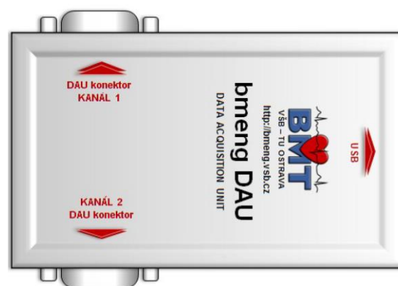
Fig. 4: Data acquisition unit (DAU).
