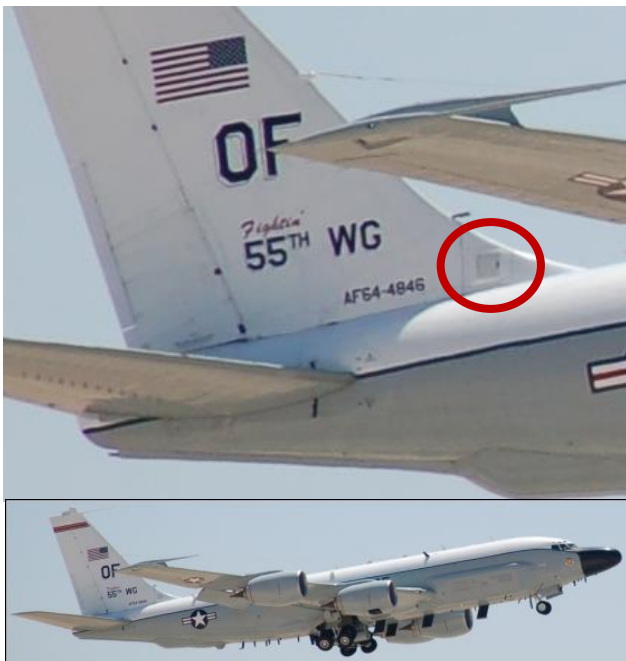
Figure 4. DFIRS in RC – 135 is flush-mounted into the vertical fin [source: http://blog.trentonsystems.com/small-footprint-rackmount-systems-airborne-surveillance/ ]
