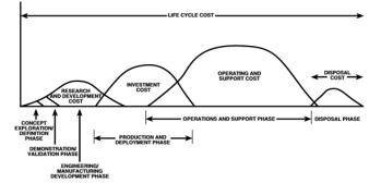
**Figure 3.** Illustration of Life Cycle Cost and its cost elements (cost categories) relating to stages/phases of a system life cycle [8].
