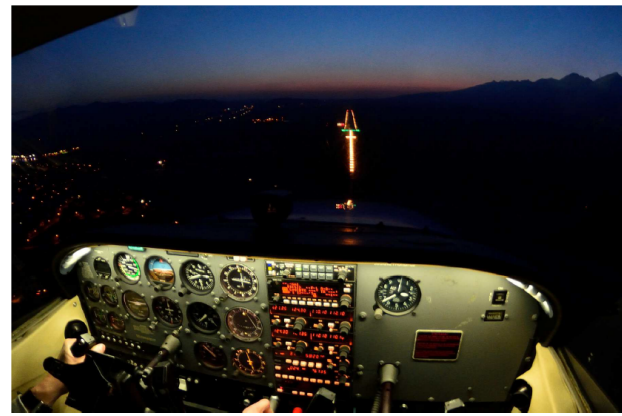
Figure 7. Final approach, PAPI are clearly visible [11].
