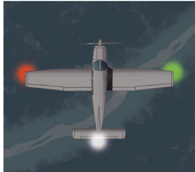
Figure 4. Aircraft position lights [11].
